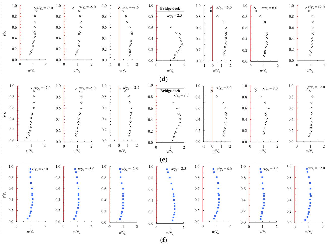
**Figure 6.** Vertical distributions of the nondimensional mean streamwise velocity  $u/V_a$  at centerline of the channel and at different nondimensional streamwise distances  $x/y_a$ ,  $F_a^* = 0.236$  and at: (a)  $y_b/y_a = 0.35$ ; (b)  $y_b/y_a = 0.55$ ; (c)  $y_b/y_a = 0.65$ ; (d)  $y_b/y_a = 0.75$ ; (e)  $y_b/y_a = 0.80$ ; and (f)  $y_b/y_a = 1.00$  (no deck).
