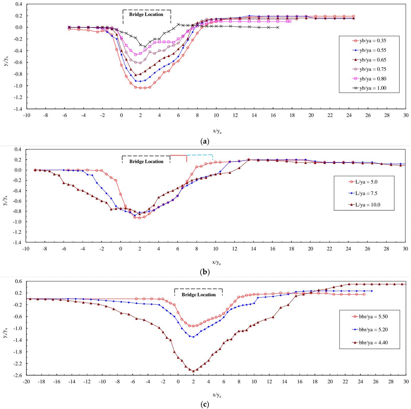
**Figure 7.** Relative scour depth  $y_s/y_a$  in the nondimensional streamwise distance  $x/y_a$  for  $F_a^* = 0.236$  and for: (a) different relative bridge opening  $y_b/y_a$ ; (b) different relative bridge lengths  $L/y_a$  and  $y_b/y_a = 0.55$ ; and (c) different relative bridge widths ( $b_{br}/y_a$ ) and  $y_b/y_a = 0.55$ .
